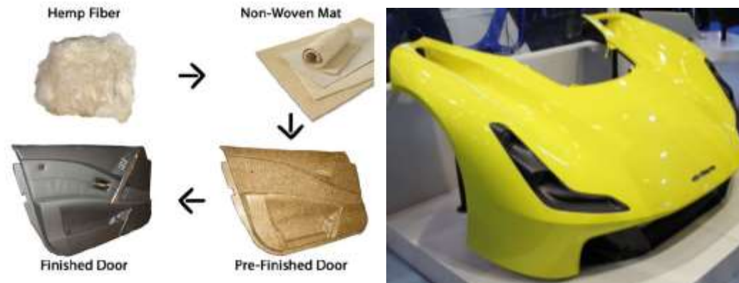
Figure 2: (a) Car door produced from hemp fibre (Peças, Carvalho, Salman &Leite, 2018), (b) fire- retardant fiber reinforced composite bonnet (Solvay, 2018)
