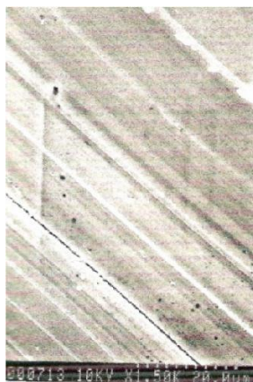
Fig. 1. SEM micrographs of Polystyrene-Cellulose acetate blends of various compositions Polystyrene/Cellulose acetate 0/100
