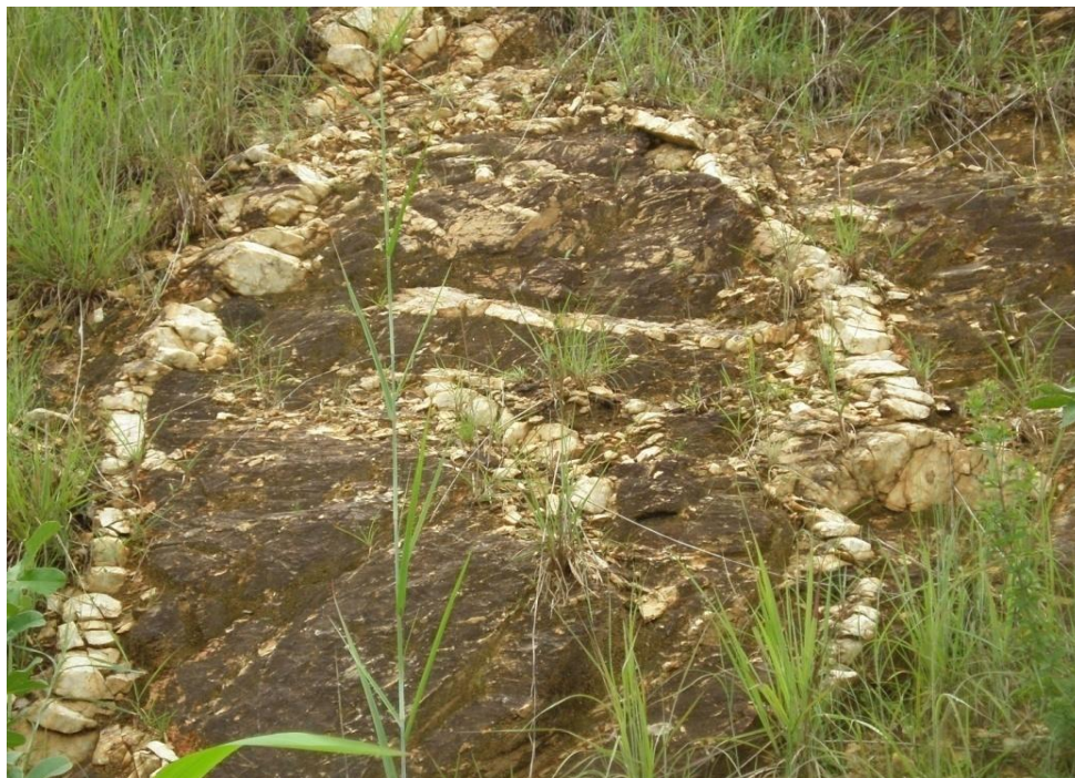
Fig. 3. Outcrop of slightly weathered schist with near vertical quartz veins (fractures) and some horizontal veins terminating against the vertical ones
