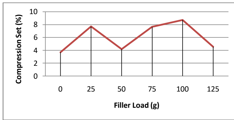
Fig. 2: Effect of filler load on compression set of the foam samples
