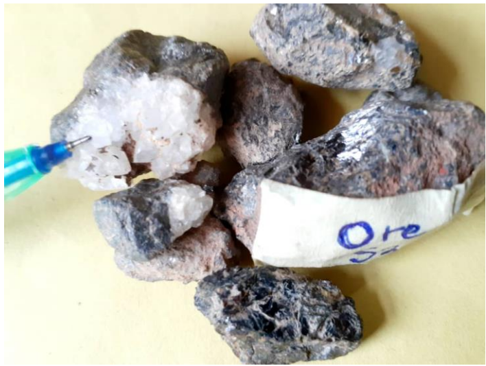
Figure 7. Ore (Pb-Zn) tailings with carbonate mineral (calcite) from Pb-Zn mining site at Iheututu area
