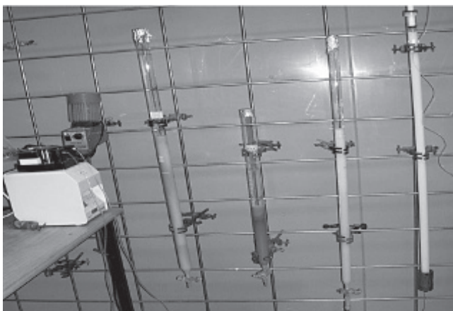
FIGURE 10.3 Open column chromatography showing the stationary phase (solid packing material).
