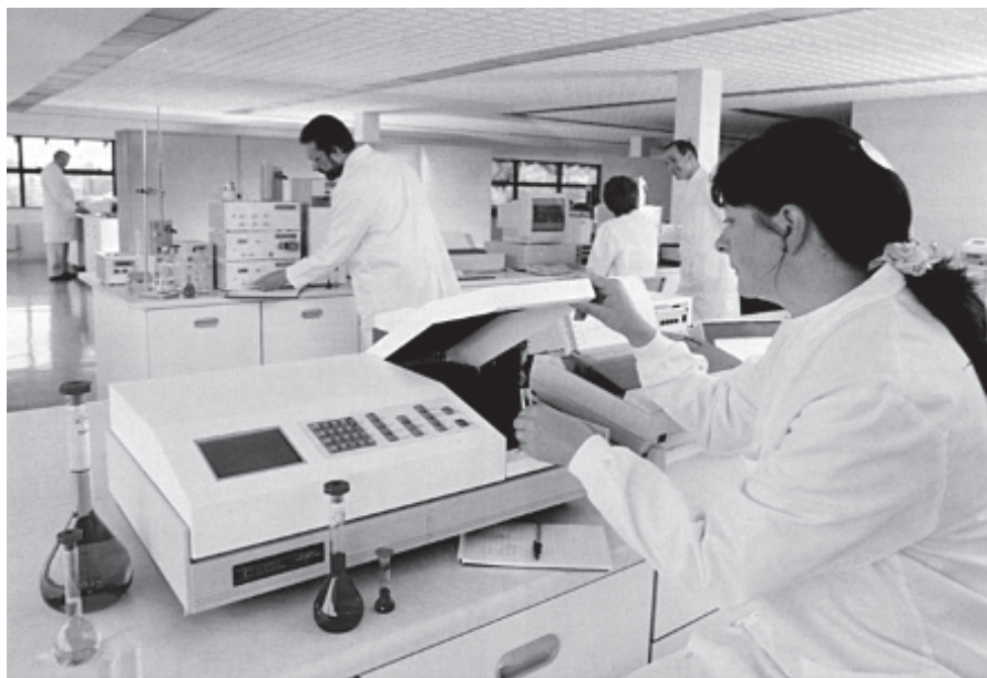
FIGURE 12.1 A typical aquarius ultraviolet/visible spectrophotometer being used within a laboratory.
