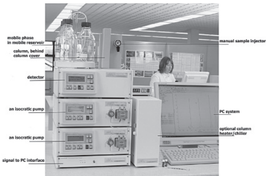
FIGURE 12.18 HPLC system components.
